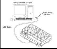
iTM for PC/Laptop to communicate with all 12 Radios inserted into the MUC through integrated USB Hub. Complies with the USB 2.0 Standard. Requires one USB A to USB micro-B cable (CB000458A07) to connect to PC. Please refer to the figure of "Connecting radios to iTM Proxy using MUC"
